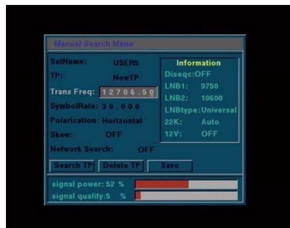
STEP 6 Using Remote Control – enter the numbers "127065" (no dot required to enter after 6)
