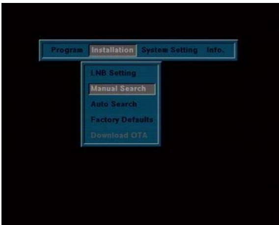
STEP 3 Using the down button go to "Manual Search" and click "OK" button
