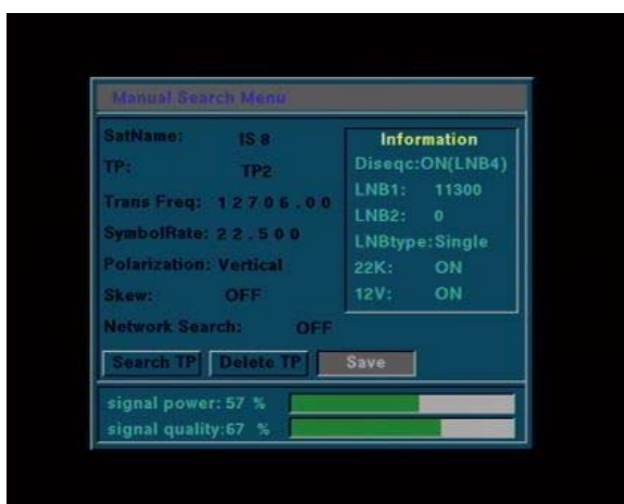
STEP 11 Using down arrow key go to "SAVE" and click OK on the Remote Control
